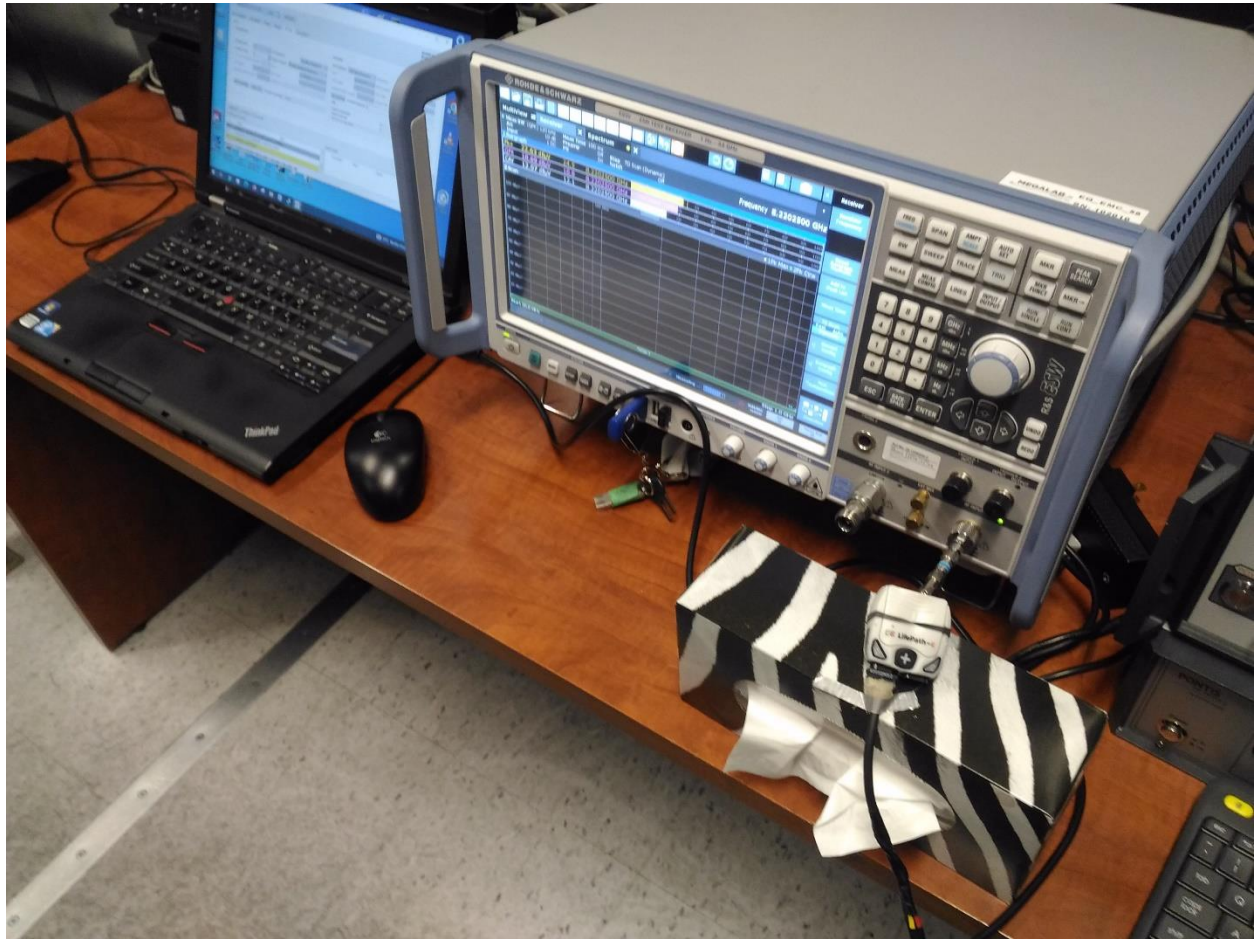
Figure 7 – Antenna Conducted Measurement Setup
