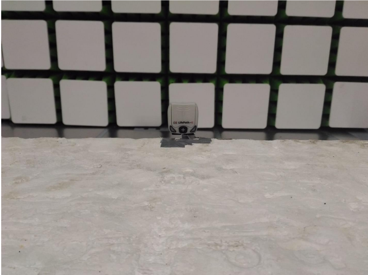
Figure 1 – Radiated Emissions Setup (Worst case orientation as tested)
