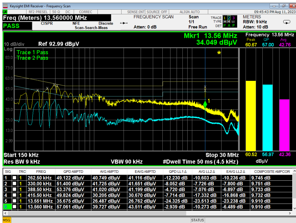
Figure 7 – Conducted Emissions Plot, Neutral, NFC, 12% RFID duty cycle, SN 0077 power supply
