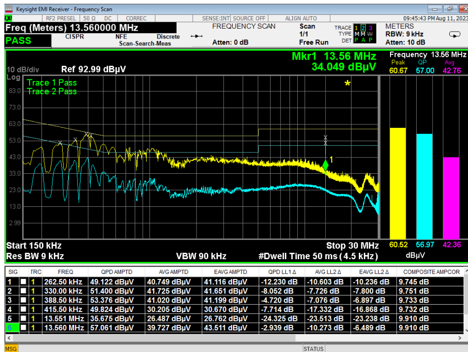
Figure 18 - Conducted Emissions, Neutral, 12% duty cycle, NCEE power supply SN 00077
