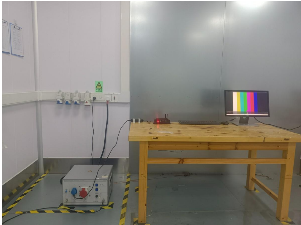
Conducted Emission at AC power line
