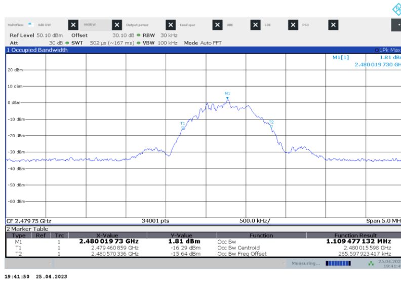
Figure 7.5-6: 99% occupied bandwidth on high channel
