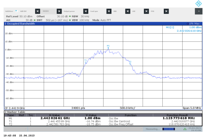
Figure 7.5-5: 99% occupied bandwidth on mid channel
