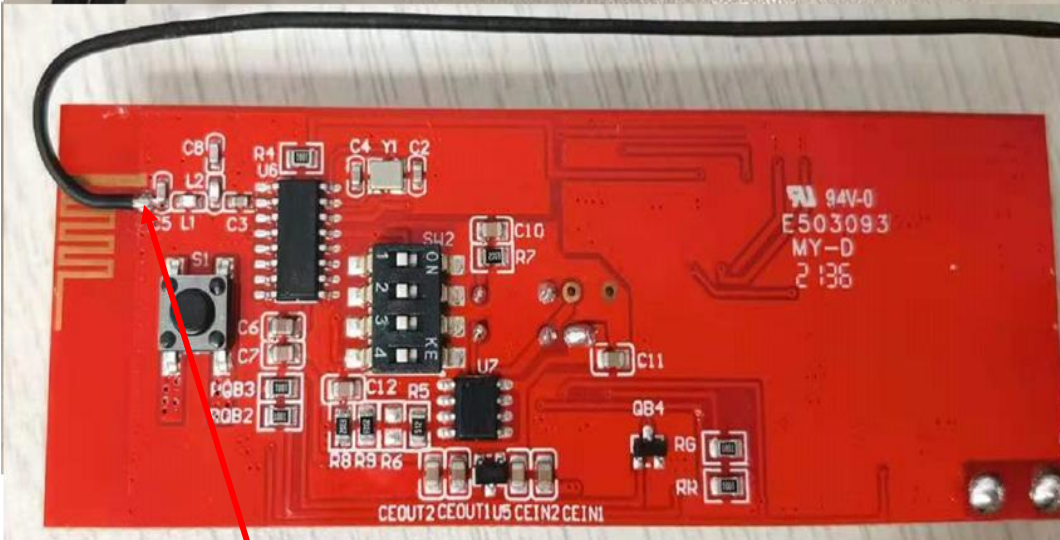
PCB antenna and wire antenna share the same antenna location
