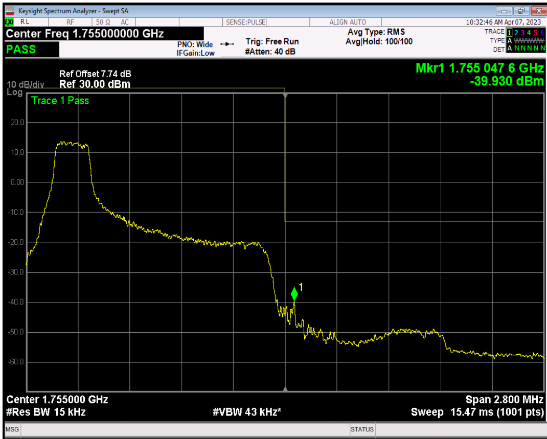
Band4 QAM16 BW=1.4MHz Channel=20393 RB Size=1 Position=#Max
