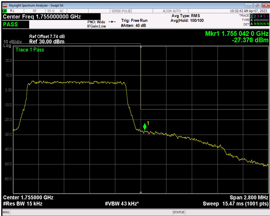
Band4 QPSK BW=1.4MHz Channel=20393 RB Size=6 Position=#0
