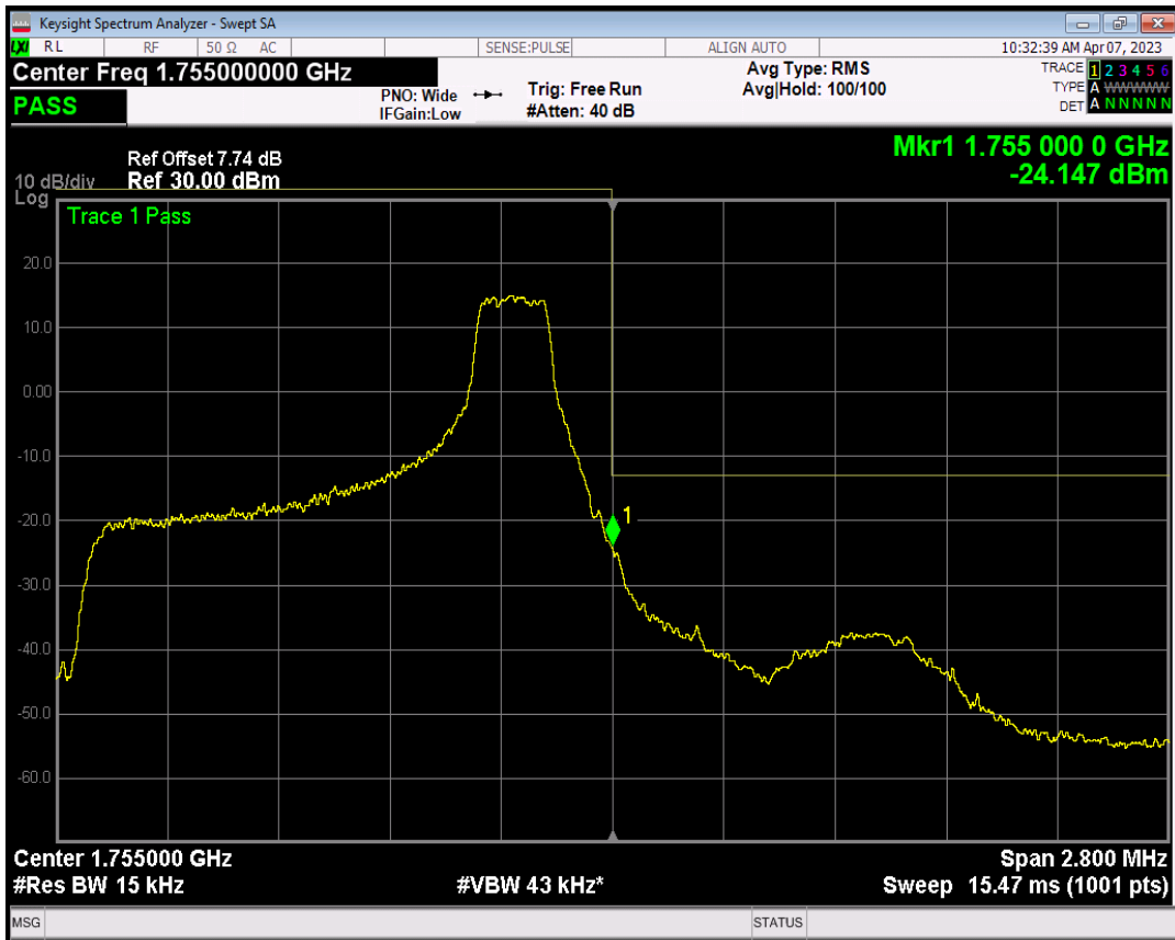
Band4 QPSK BW=1.4MHz Channel=20393 RB Size=6 Position=#0
