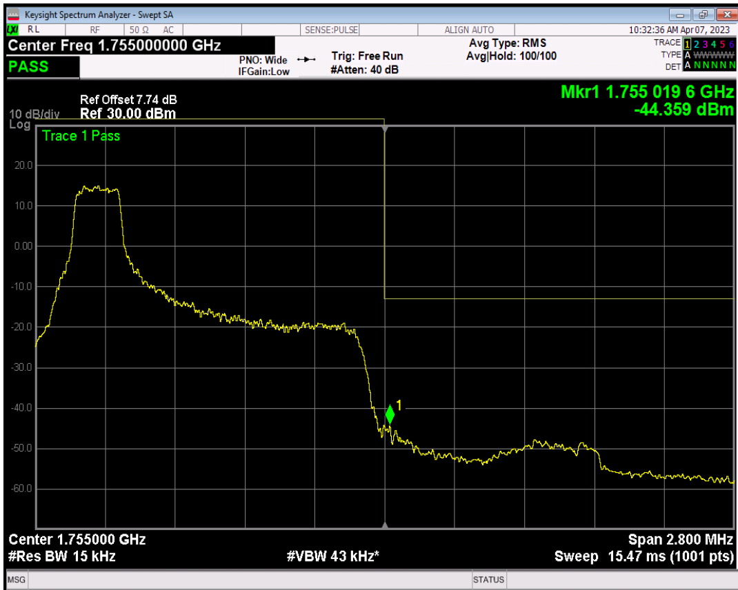
Band4 QPSK BW=1.4MHz Channel=20393 RB Size=1 Position=#0
