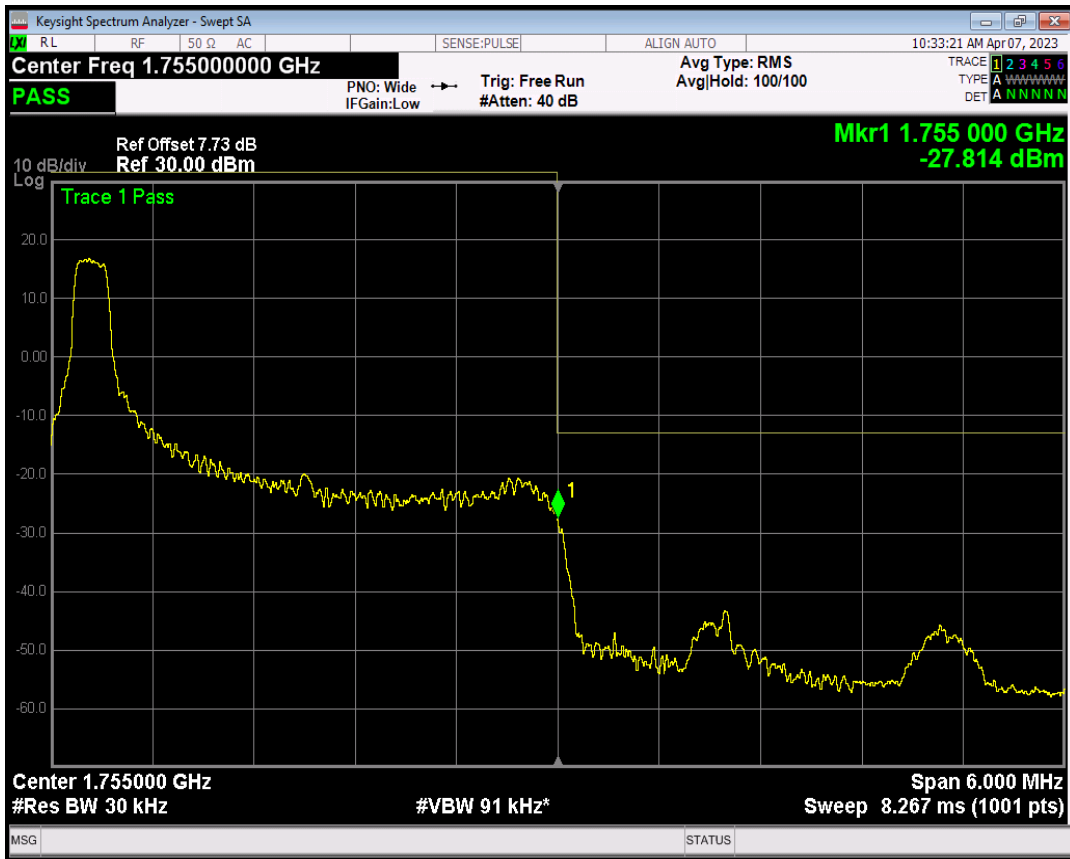
Band4 QAM16 BW=3MHz Channel=20385 RB Size=1 Position=#Max
