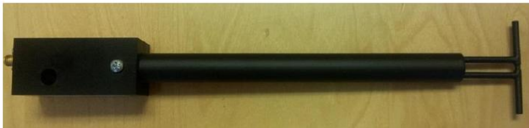
Figure 1 – MVG COMOSAR Validation Dipole
