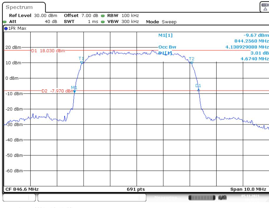
**26 dB Emissions &99% Occupied Bandwidth for HSUPA (BPSK) Mode, Low channel**
