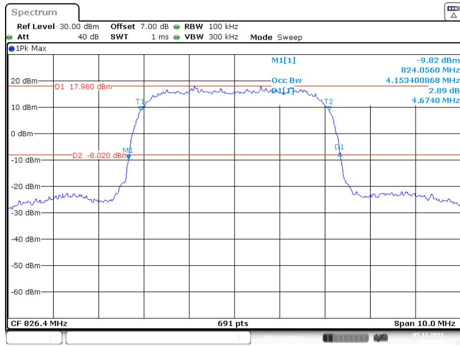
**26 dB Emissions &99% Occupied Bandwidth for RMC (BPSK) Mode, Middle channel**
