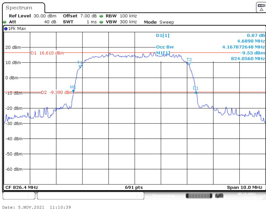
**26 dB Emissions &99% Occupied Bandwidth for HSDPA (16QAM) Mode, Middle channel**
