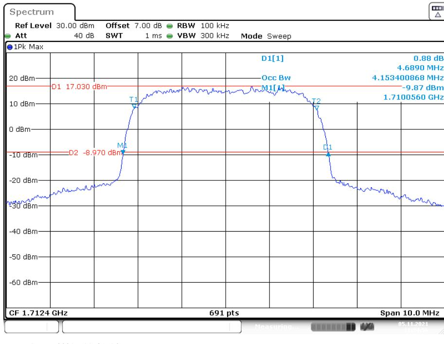
**26 dB Emissions &99% Occupied Bandwidth for HSUPA (BPSK) Mode, Middle channel**
