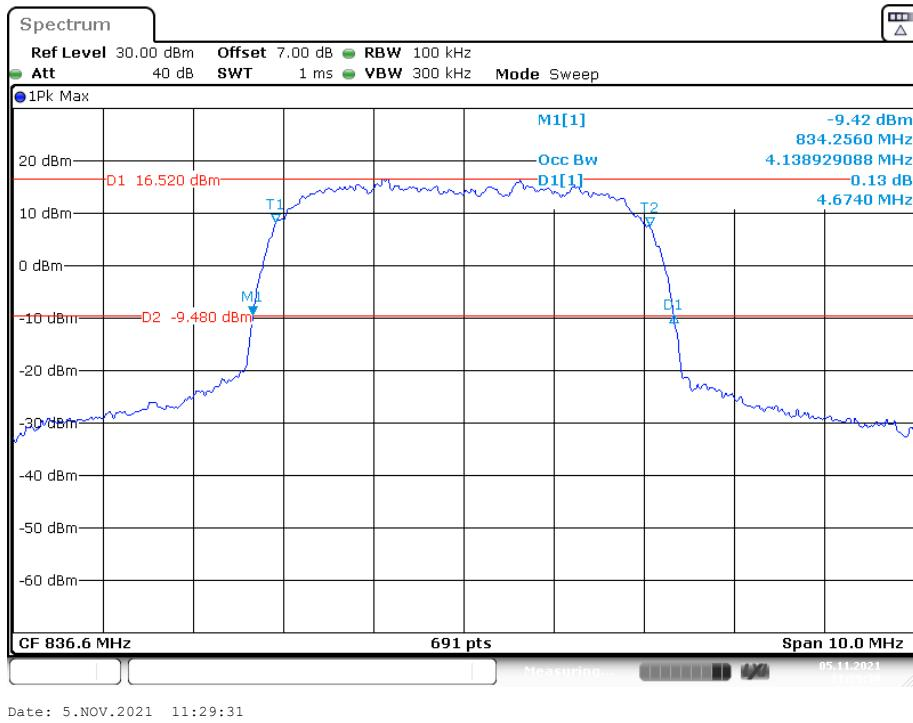
**26 dB Emissions &99% Occupied Bandwidth for HSUPA (BPSK) Mode, High channel**
