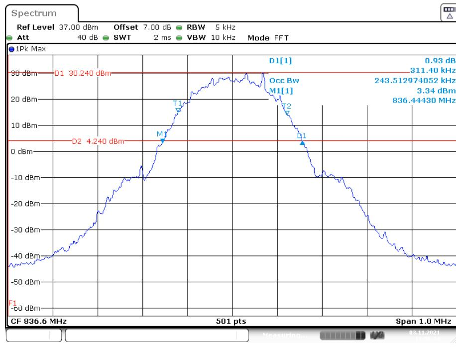
**26 dB Emissions &99% Occupied Bandwidth for GSM (GMSK) Mode, High channel**
