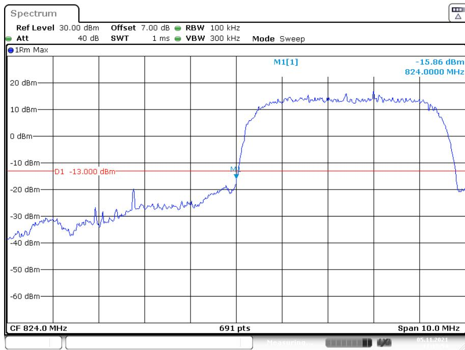
**Cellular Band, Right Band Edge for HSDPA (16QAM) Mode**
