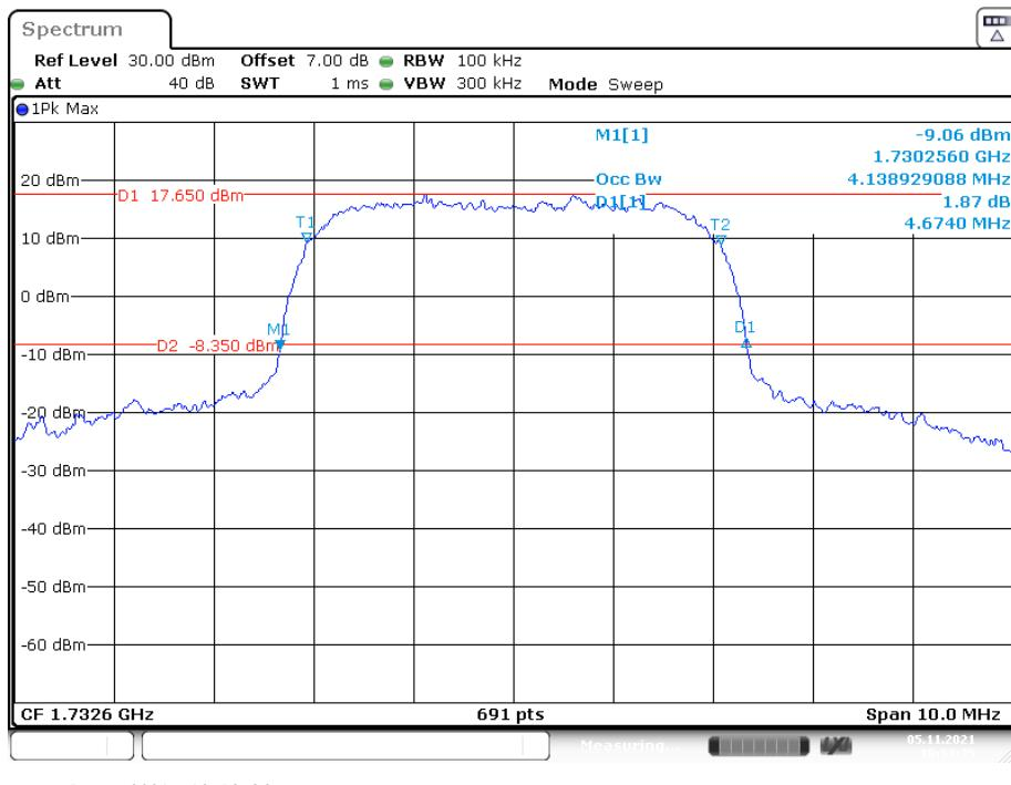
**26 dB Emissions &99% Occupied Bandwidth for RMC (BPSK) Mode, High channel**
