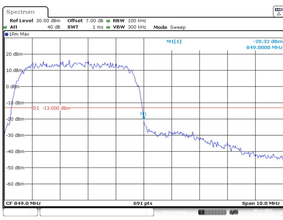
**Cellular Band, Left Band Edge for HSDPA (16QAM) Mode**
