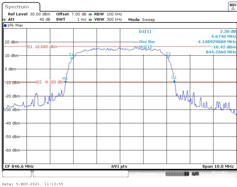
**PCS Band (Part 24E)****26 dB Emissions &99% Occupied Bandwidth for GSM (GMSK) Mode, Low channel**
