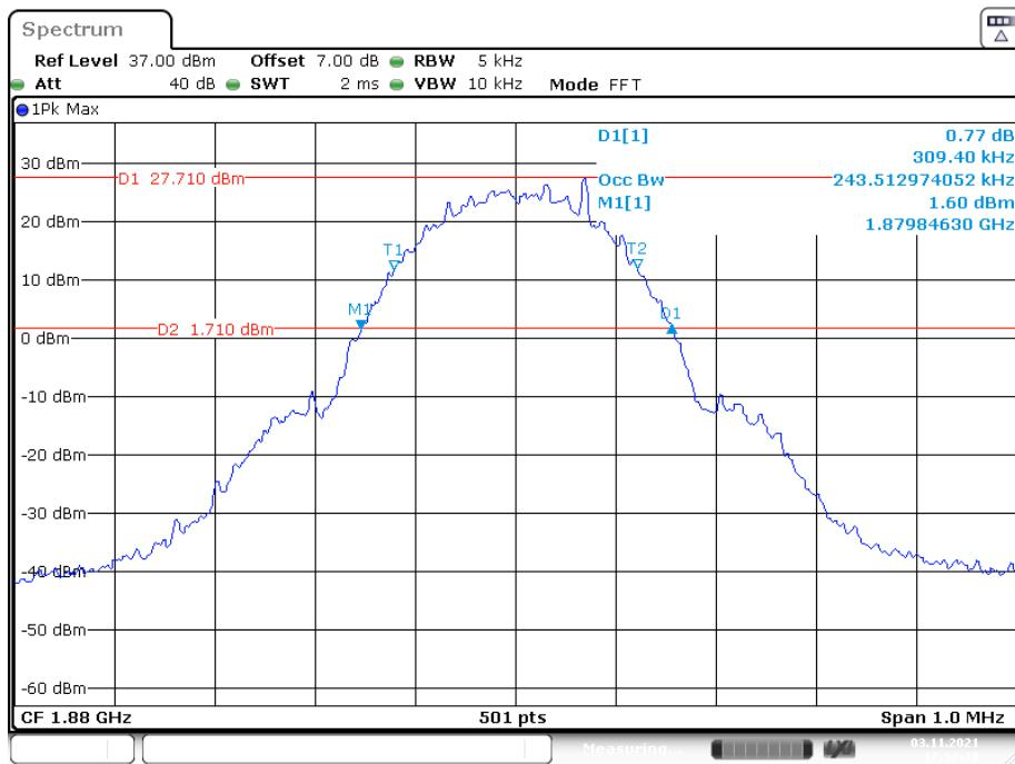
**26 dB Emissions &99% Occupied Bandwidth for GSM (GMSK) Mode, High channel**
