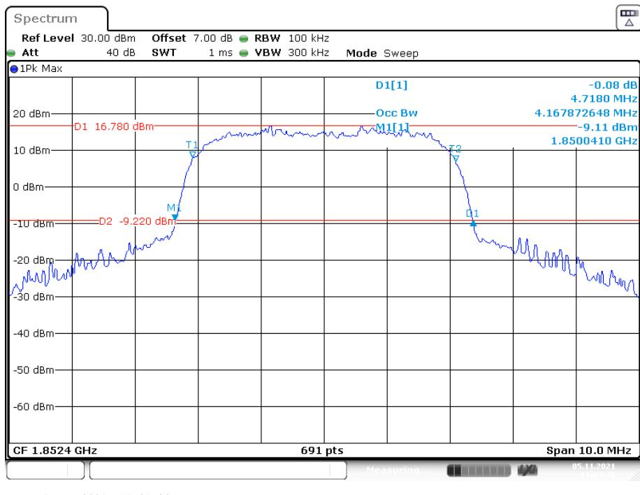
**26 dB Emissions &99% Occupied Bandwidth for HSDPA (16QAM) Mode, Middle channel**
