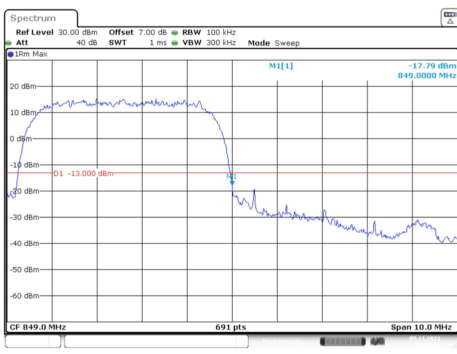
**Cellular Band, Left Band Edge for HSUPA (BPSK) Mode**
