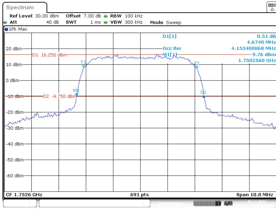
**26 dB Emissions &99% Occupied Bandwidth for HSDPA (16QAM) Mode, Low channel**
