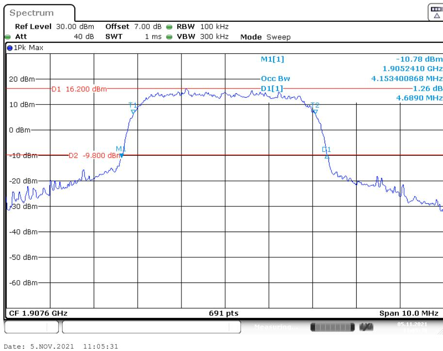
**AWS Band (Part 27)****26 dB Emissions &99% Occupied Bandwidth for RMC (BPSK) Mode, Low channel**
