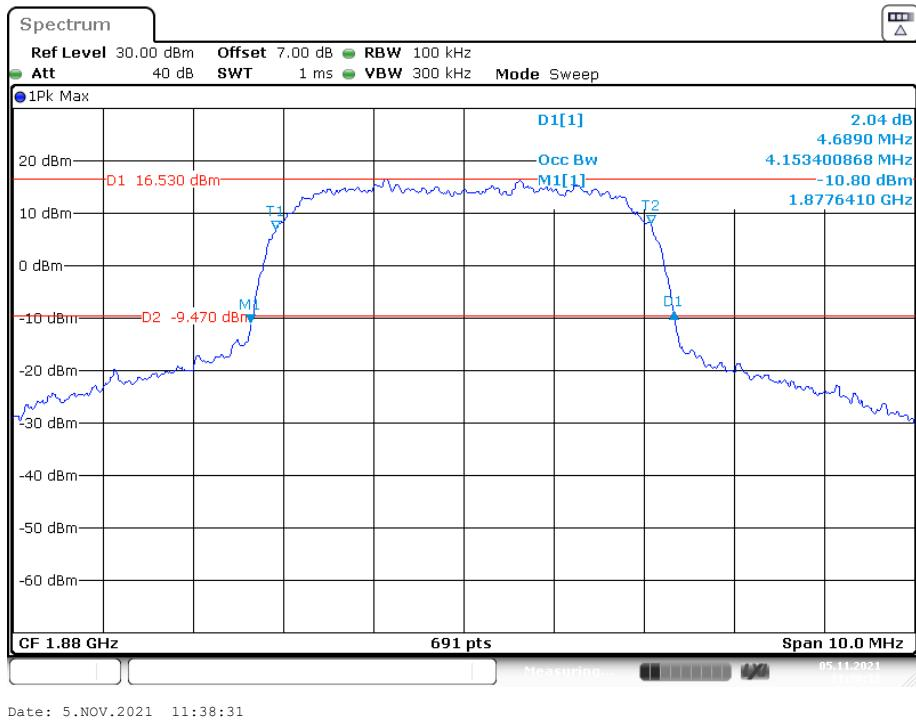
**26 dB Emissions &99% Occupied Bandwidth for HSUPA (BPSK) Mode, High channel**
