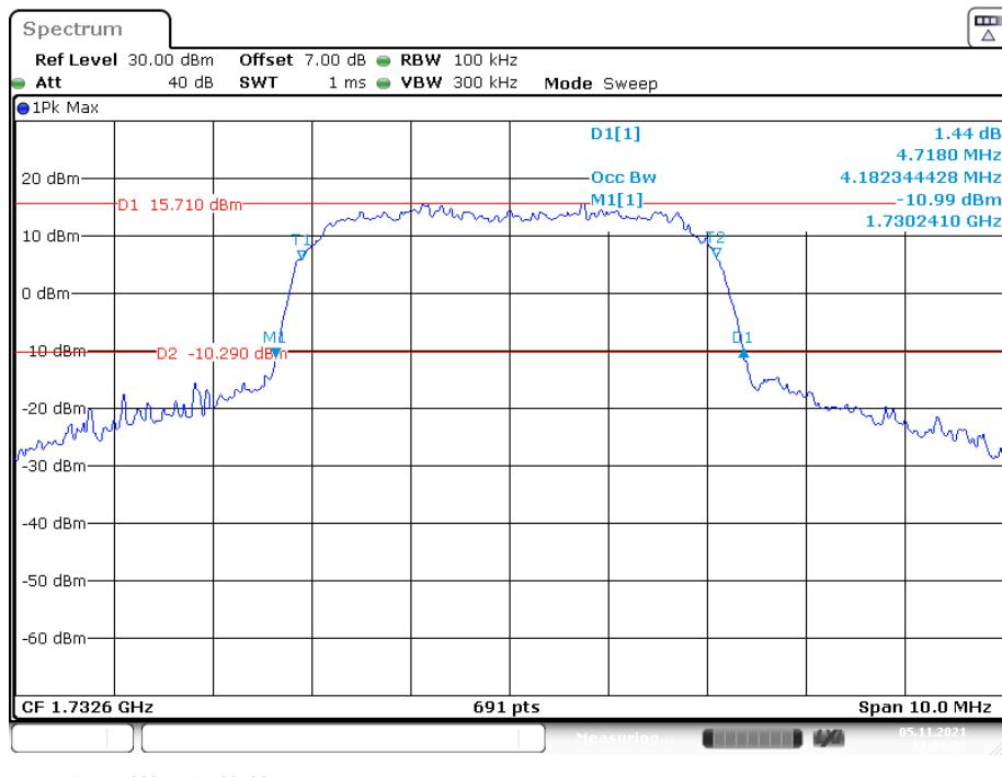
**26 dB Emissions &99% Occupied Bandwidth for HSDPA (16QAM) Mode, High channel**
