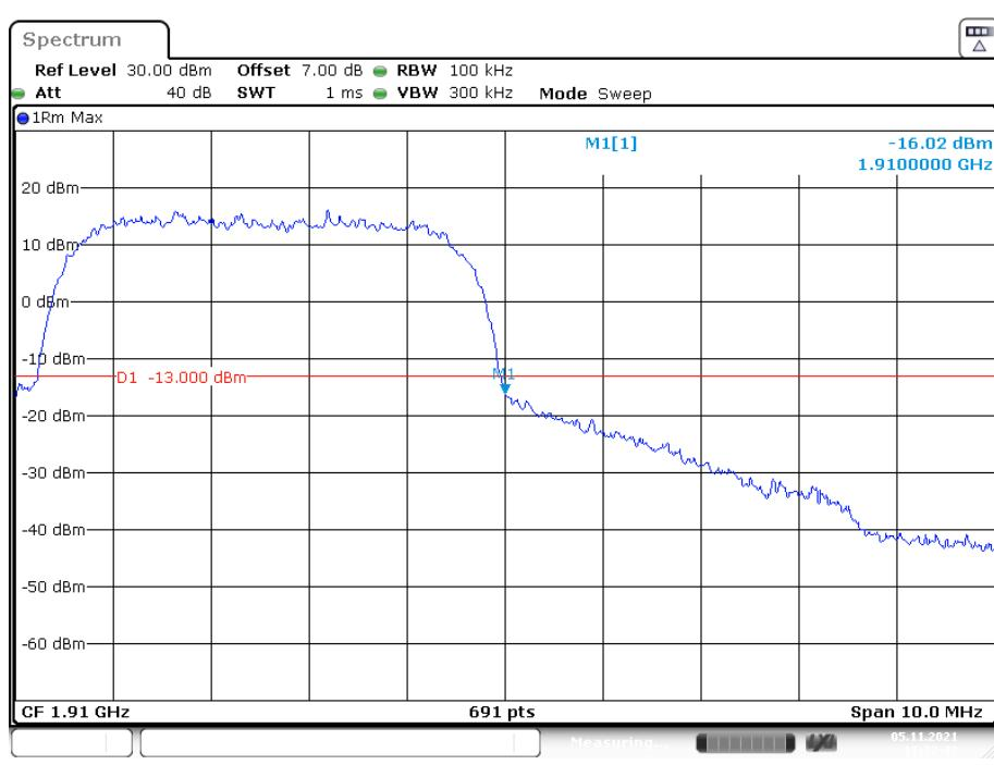
**AWS Band, Left Band Edge for RMC (BPSK) Mode**
