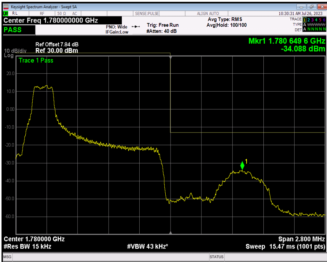
Band66 QPSK BW=1.4MHz Channel=132665 RB Size=1 Position=#Max
