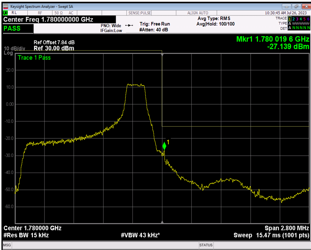
Band66 16QAM BW=1.4MHz Channel=132665 RB Size=6 Position=#0
