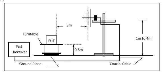
(c) For radiated emissions above 1000MHz
