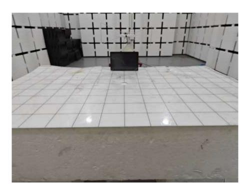
Set-up for Radiated Emission (RE), Above 1GHz
