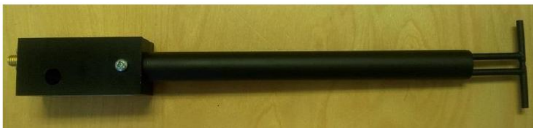
Figure 1 – MVG COMOSAR Validation Dipole
