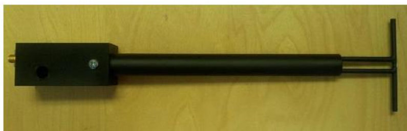
Figure 1 – MVG COMOSAR Validation Dipole
