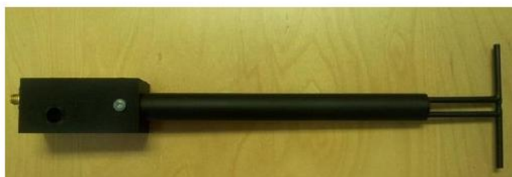
Figure 1 – MVG COMOSAR Validation Dipole
