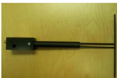
Figure 1 – MVG COMOSAR Validation Dipole
