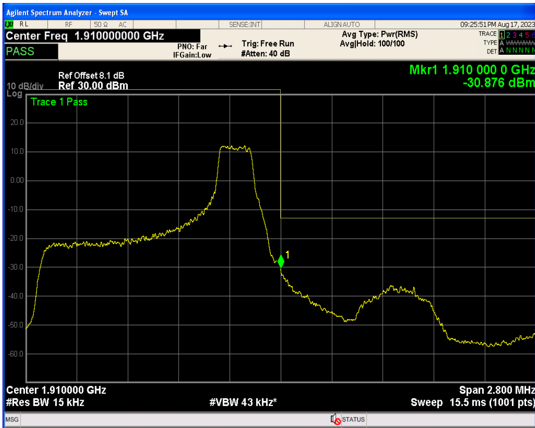
Band2 QPSK BW=3MHz Channel=18615 RB Size=1 Position=#0
