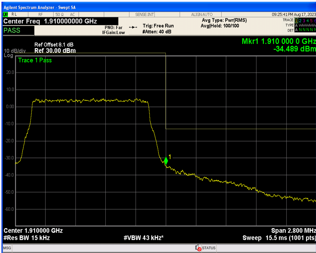
Band2 16QAM BW=1.4MHz Channel=19193 RB Size=1 Position=#0
