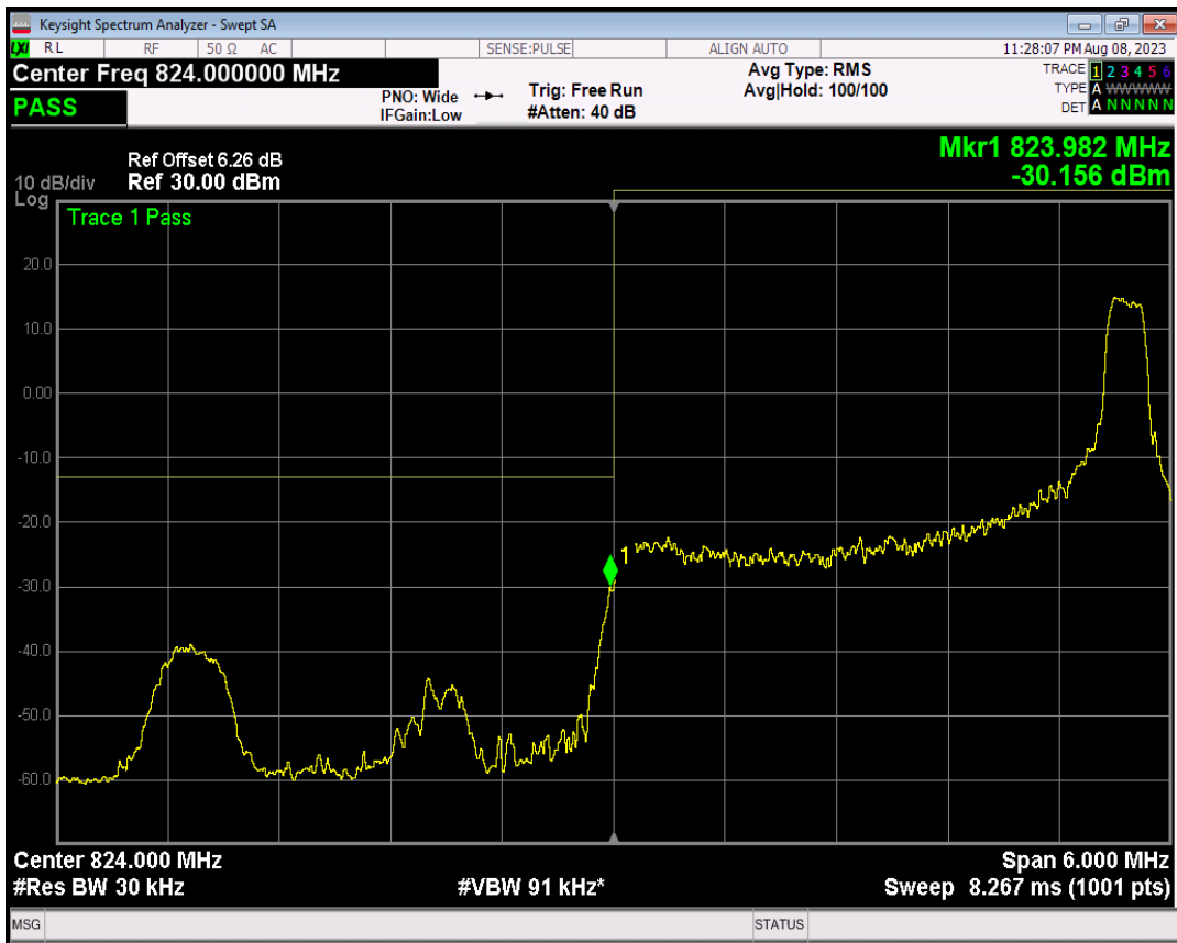
Band5 16QAM BW=3MHz Channel=20415 RB Size=15 Position=#0
