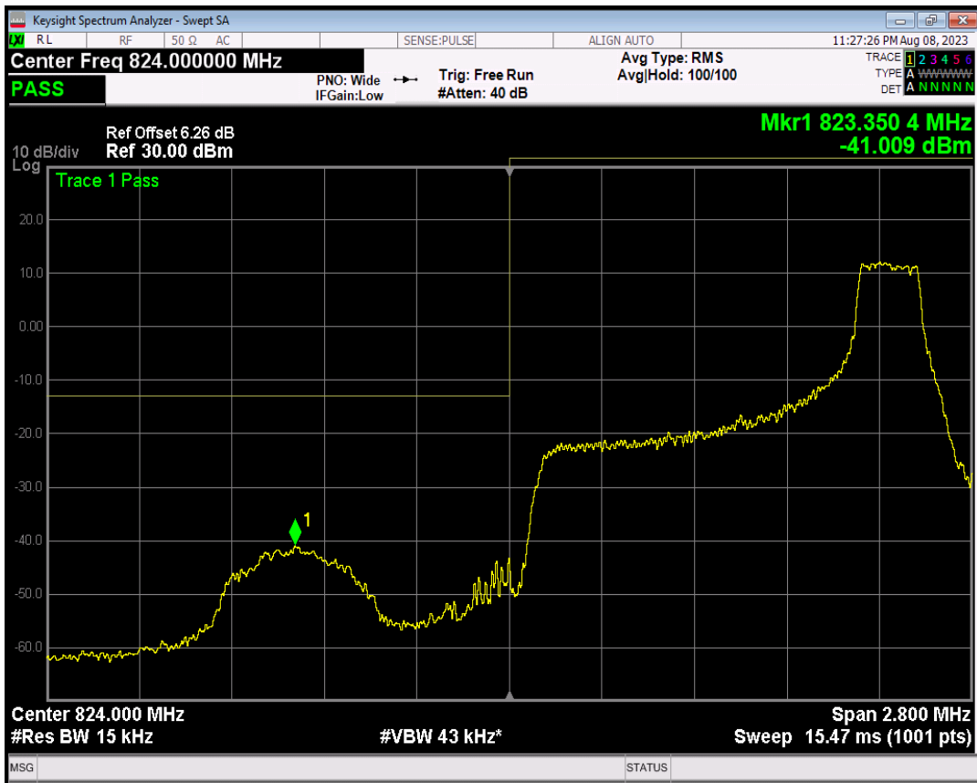
Band5 16QAM BW=1.4MHz Channel=20407 RB Size=6 Position=#0
