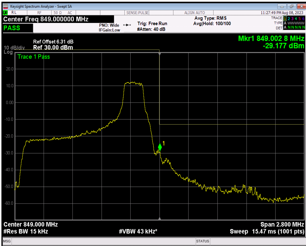
Band5 16QAM BW=1.4MHz Channel=20643 RB Size=6 Position=#0
