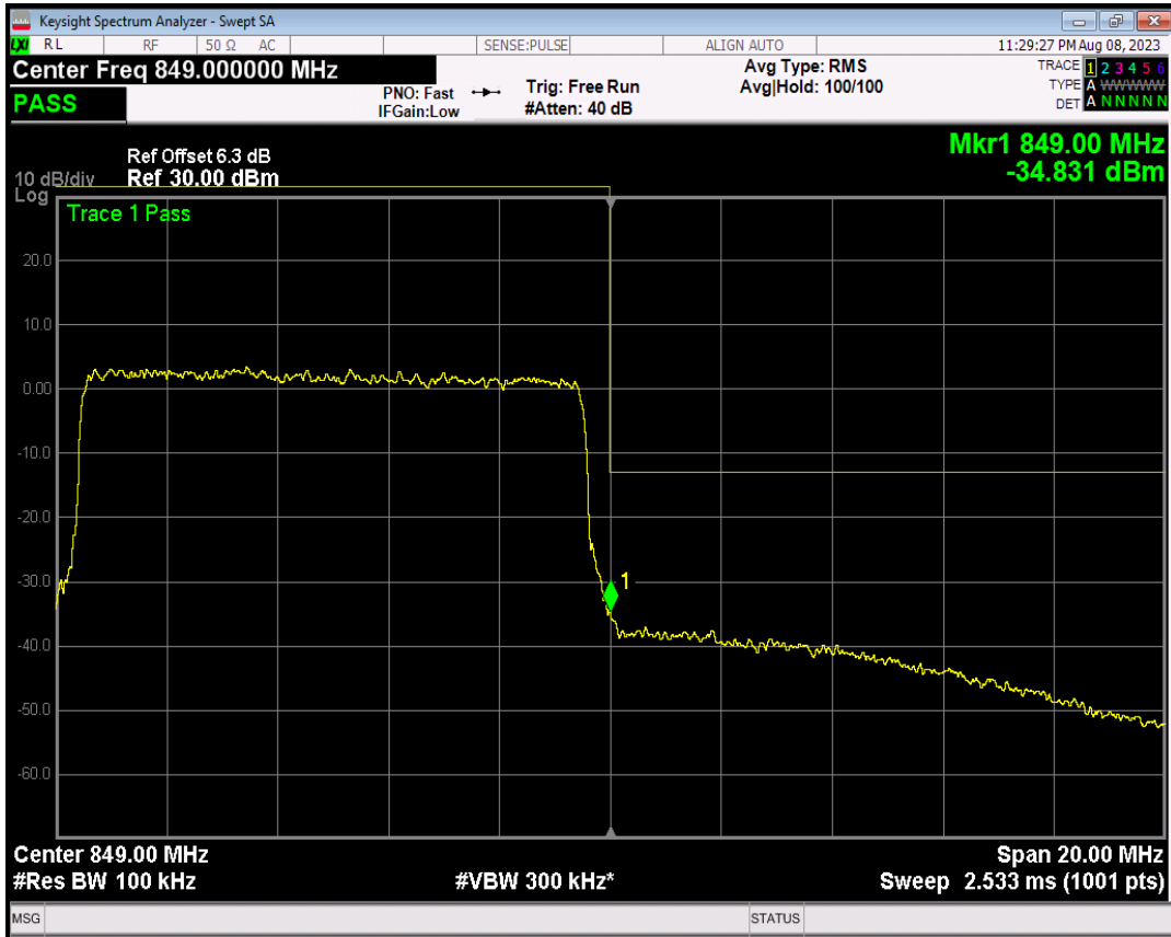
Band66 QPSK BW=1.4MHz Channel=131979 RB Size=1 Position=#0
