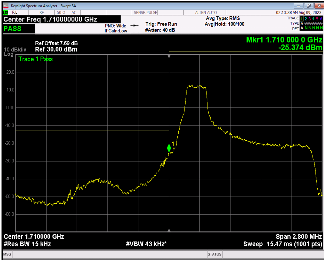
Band66 16QAM BW=1.4MHz Channel=131979 RB Size=1 Position=#Max
