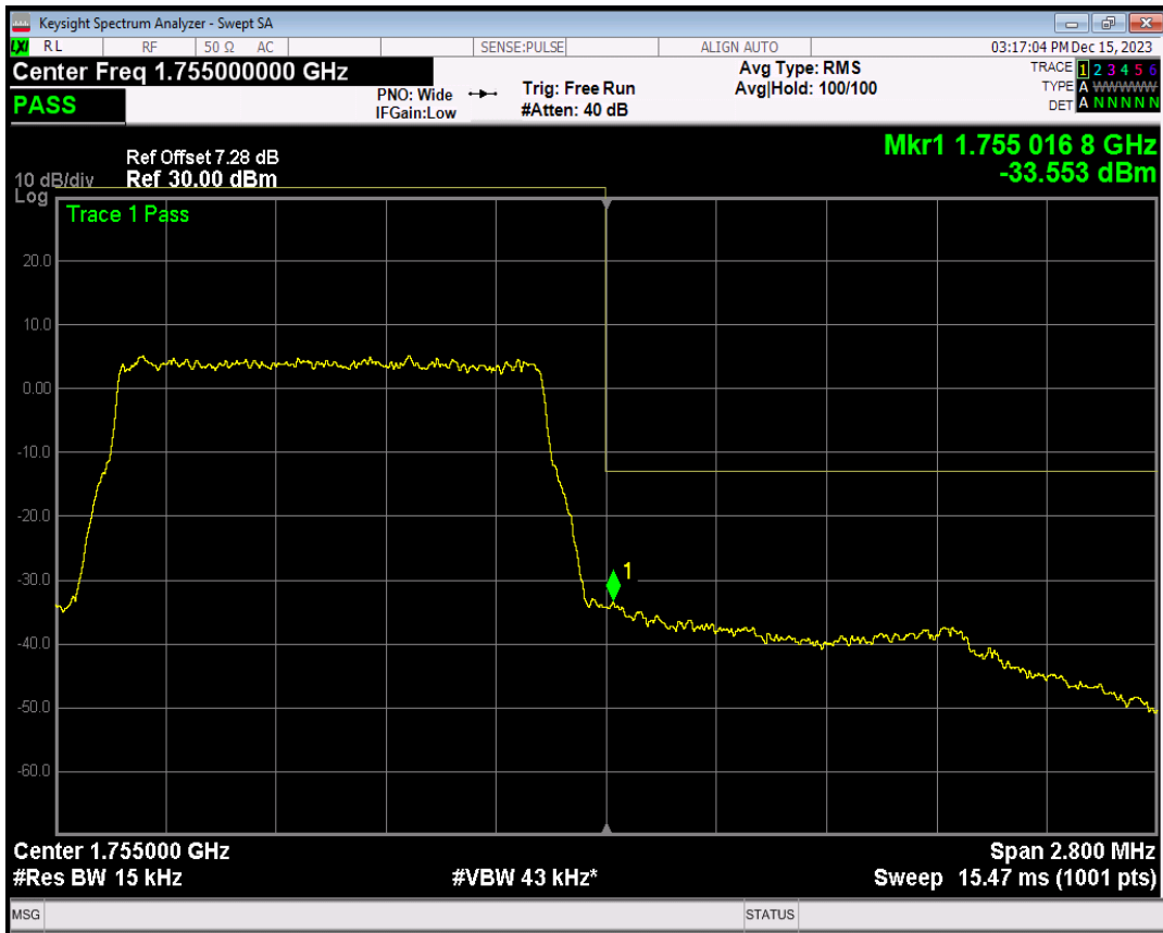
Band4 QPSK BW=1.4MHz Channel=20393 RB Size=6 Position=#0
