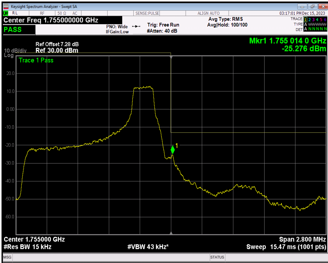
Band4 QPSK BW=1.4MHz Channel=20393 RB Size=6 Position=#0
