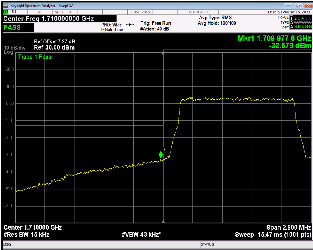
Band4 QPSK BW=1.4MHz Channel=20393 RB Size=1 Position=#0
