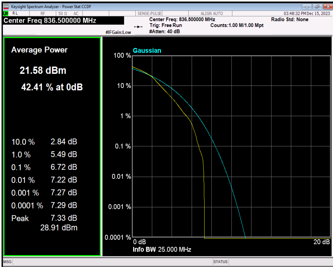
Band5 16QAM BW=10MHz Channel=20525 RB Size=1 Position=#0
