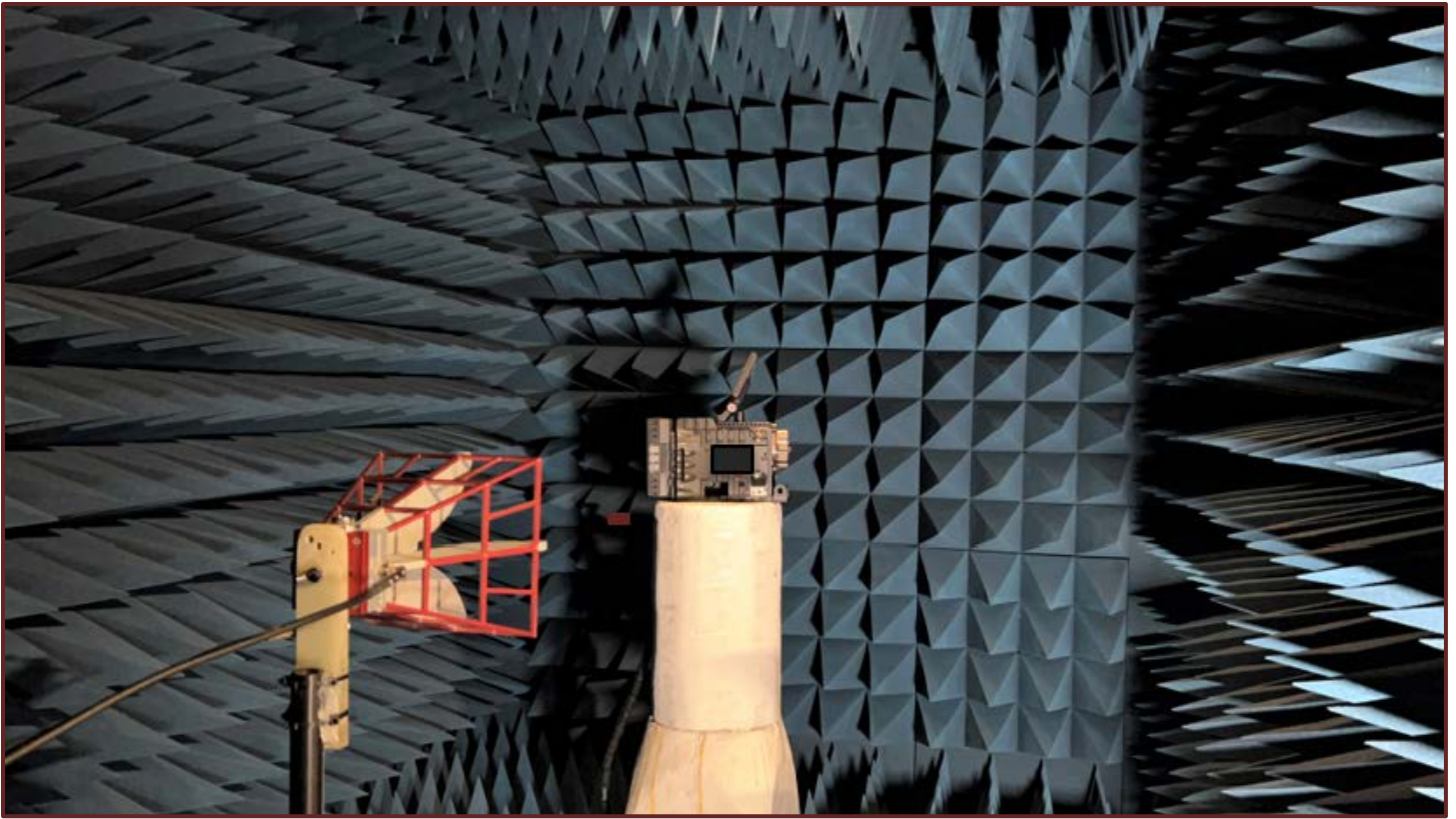
CIA's Anechoic Chamber
