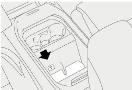
A wireless charging pad is located in the center console storage compartment.
