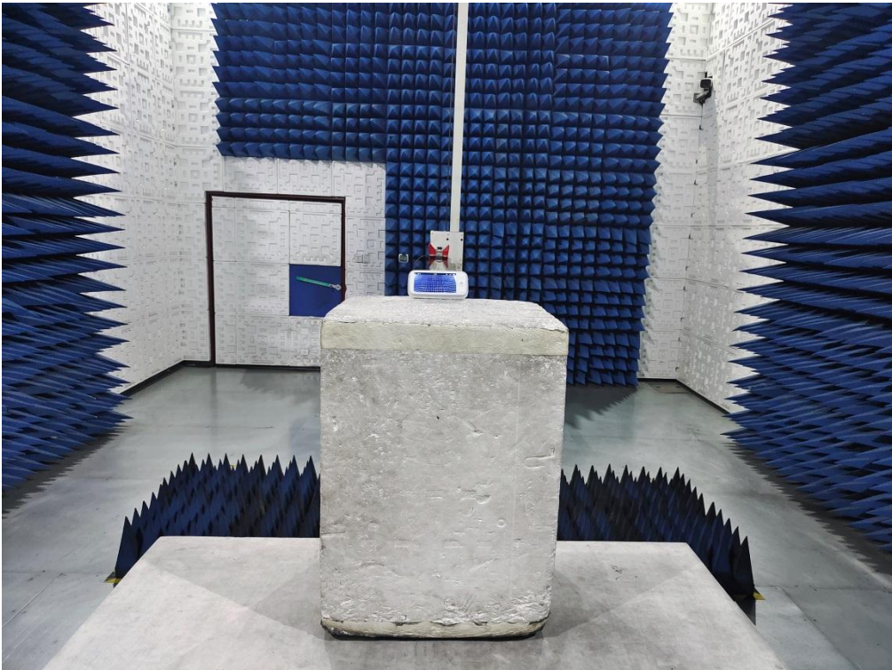
RADIATED EMISSION TEST SETUP ABOVE 1GHz
