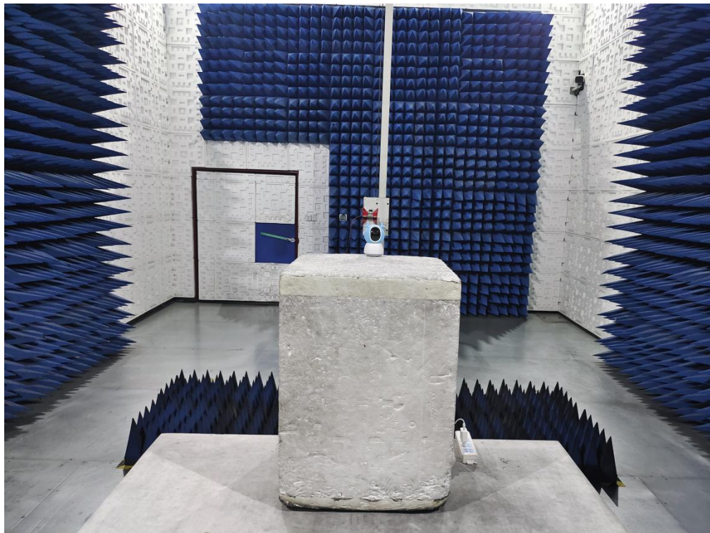
RADIATED EMISSION TEST SETUP ABOVE 1GHz
