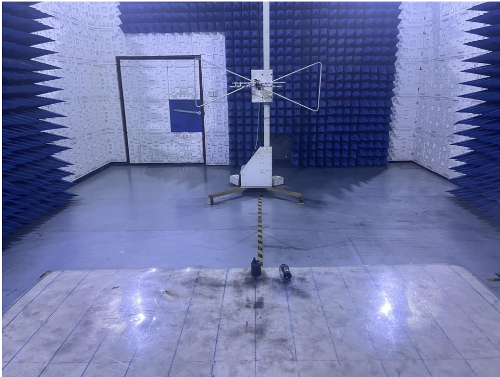
RADIATED EMISSION TEST SETUP ABOVE 1GHz
