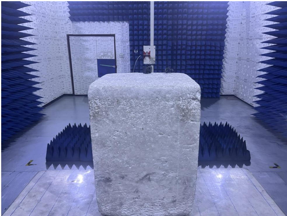
RADIATED EMISSION TEST SETUP ABOVE 1GHz
