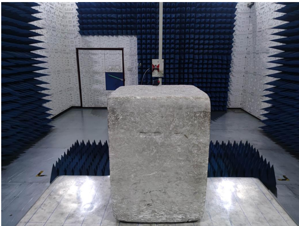
RADIATED EMISSION TEST SETUP ABOVE 1GHz
