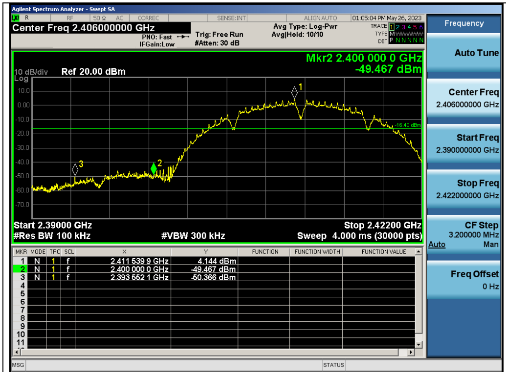
Test_Graph_802.11b_ANT1_2412_1Mbps_Lower Band Edge Emissions
