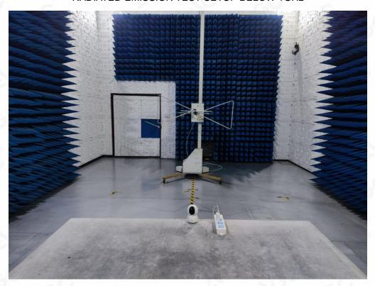
RADIATED EMISSION TEST SETUP ABOVE 1GHz
