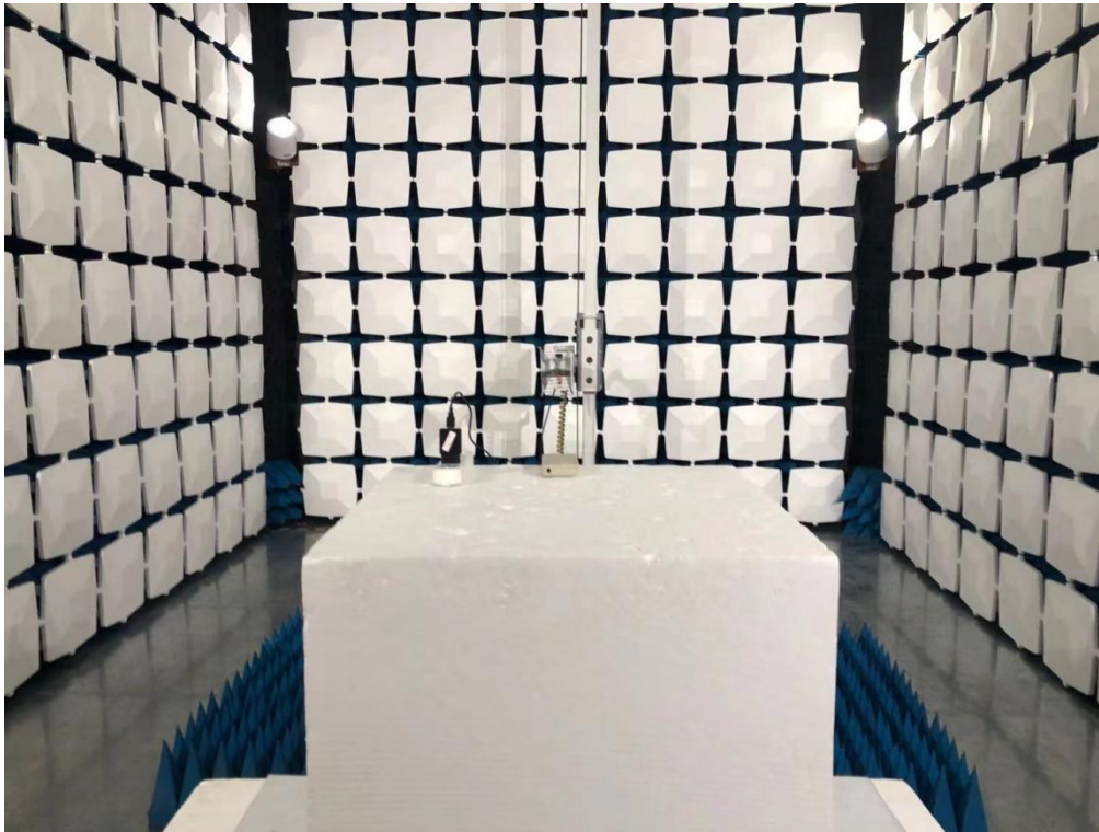
Above 1GHz for radiated emission test setup
