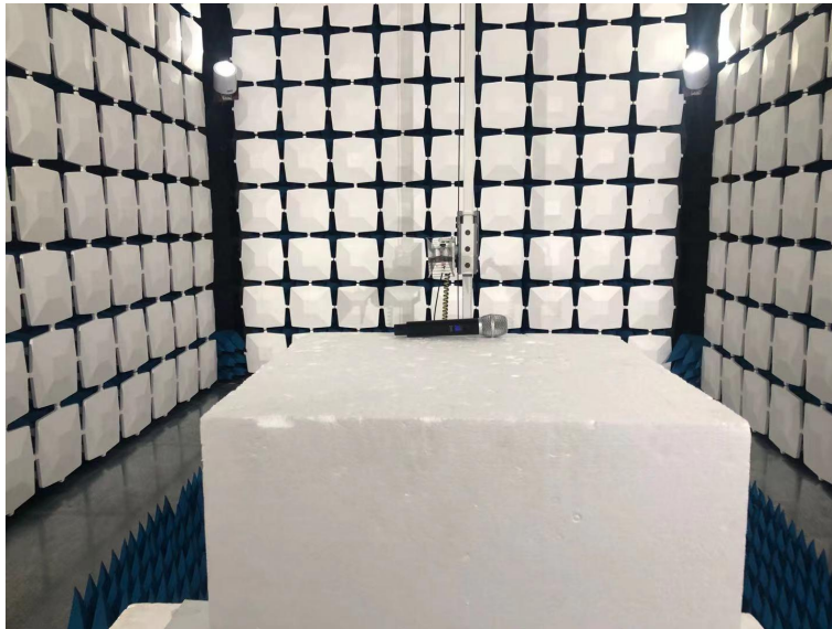
Blow 1GHz for radiated emission test setup
