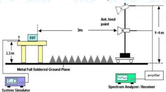
**Above 1GHz Test Setup**
