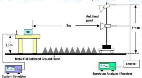
**Above 1GHz Test Setup**
