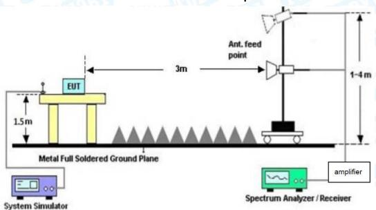
**Above 1GHz Test Setup**
