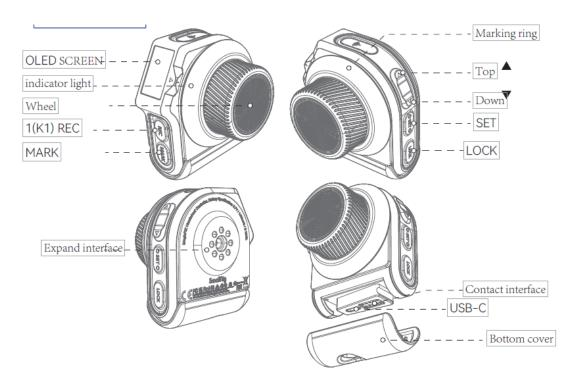
REC key: 1. Start and stop REC recording; 2. On/off function.
