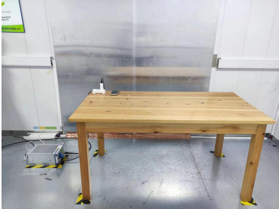
Conducted emission test setup
