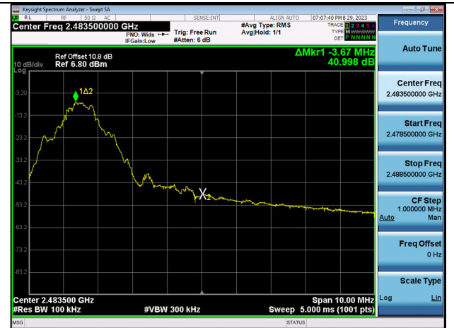
GFSK(without hopping) Band Edge(CH. 40)
