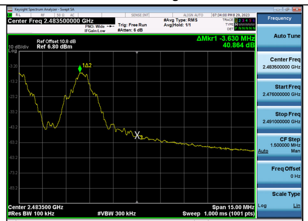
GFSK(with hopping) Band Edge
