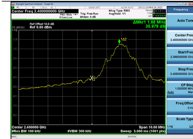
GFSK(without hopping) Band Edge(CH. 1)
