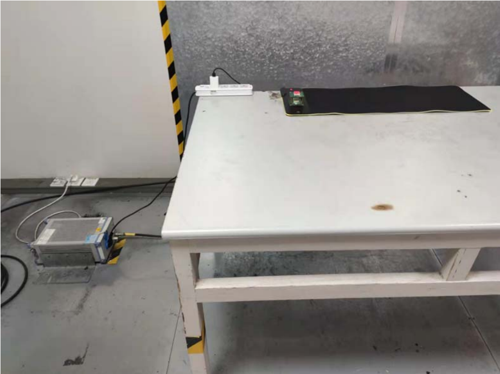
Conducted Emissions Test
