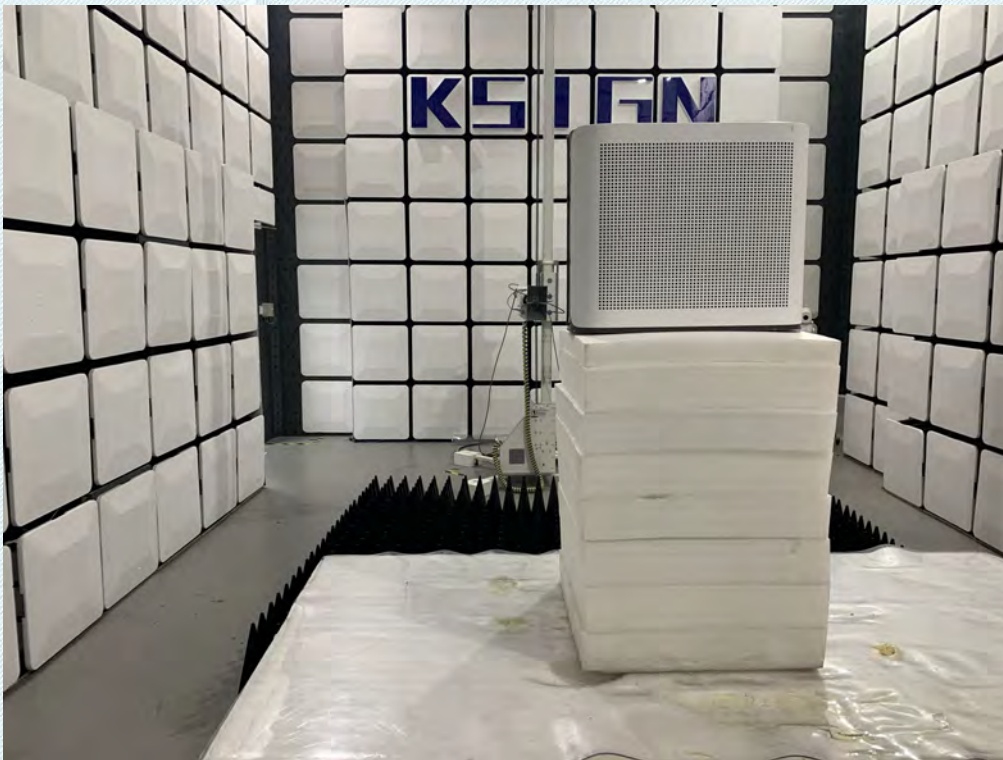
Radiated Measurement (Above 1GHz)
