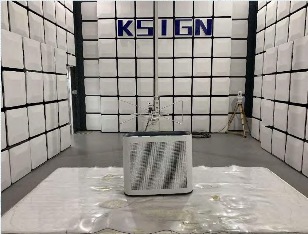
Radiated Measurement (Above 1GHz)
