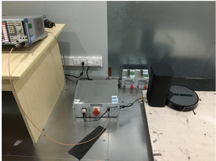
Conducted Emission Test Setup
