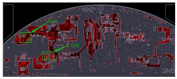
$2\sqrt{100}$  The charging IC is adjusted from sc89171 (U4) to mp26124 (U19)
