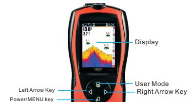
When FF1108-1CWLA powers on, the will temporarily display on screen last for 5seconds. Then will show ,From this menu, use the arrow keys to select either Start-Up, Simulator.
