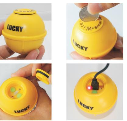
1. Press Switch 1, wireless sensor will be turned on, and working Indicator will be lit.
