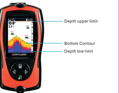
There is also a series of manual ranges which can be selected. The manual depth ranges are determined by the present depth conditions.
