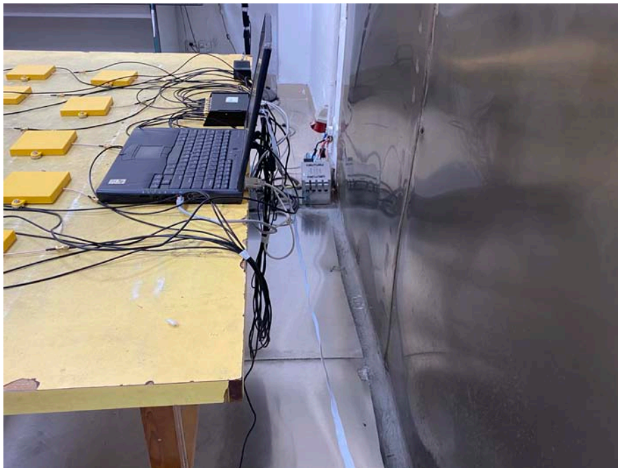
Conducted Emissions Test Setup Side View
