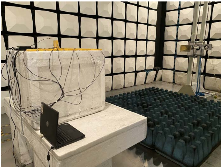
Radiated Emission Rear View (Above 1GHz)
