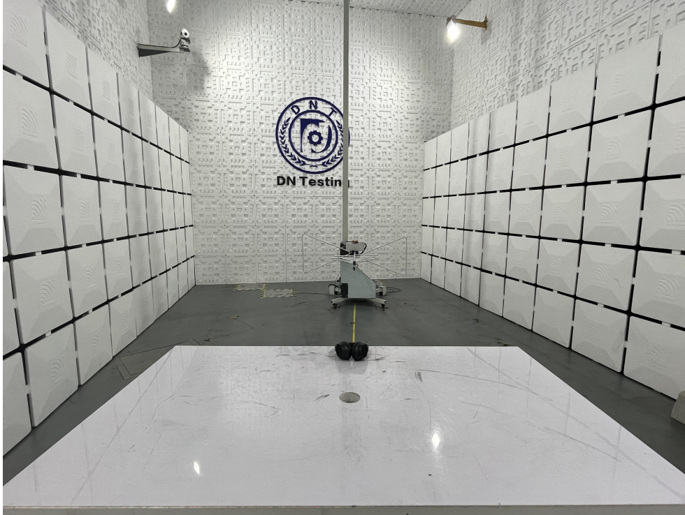
Radiated Emission Test View|(Below 1G)
