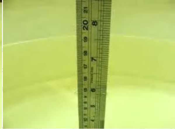
Photo of Liquid Height for Body SAR
