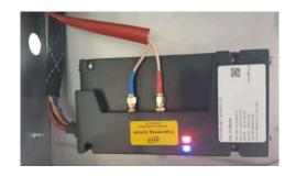
Fixing self locking hexagon nut M3 PEM M3 Power supply Cable Antenna connections
