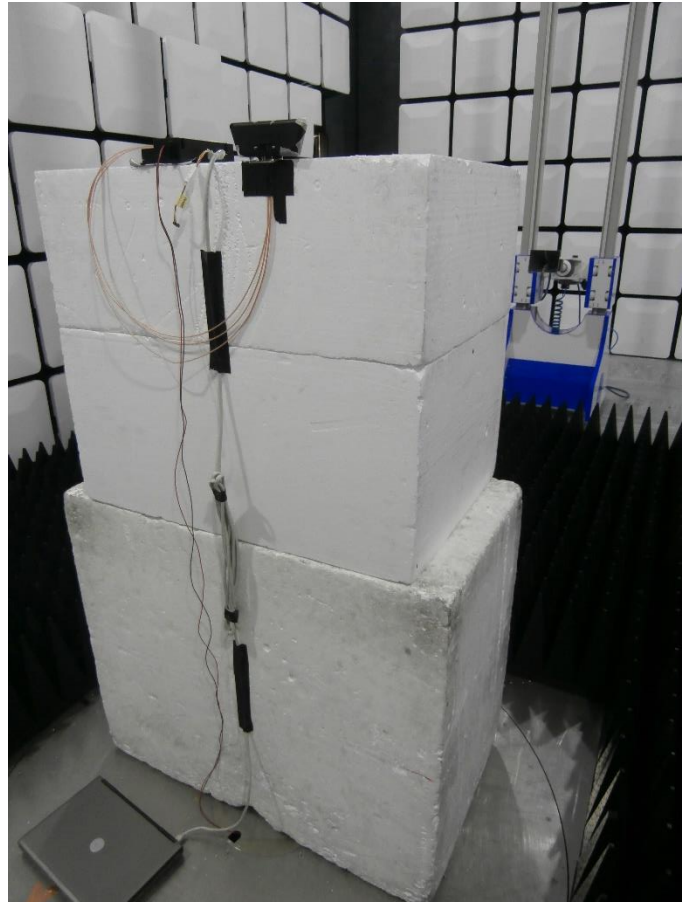
Figure 9 – Test Setup Photo, 1 GHz to 10 GHz
