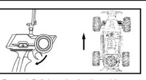
1. Forward: Pull down the throttle and then the remote control car moves forward. The moving speed can be adjusted by regulating the throttle.
