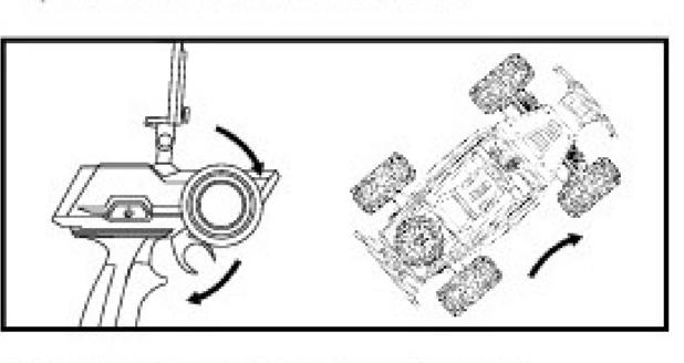
4. Turn Right Forward: Pull down the throttle and turn the right steering wheel.
