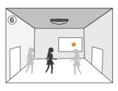
Light turn off when ambient lux level is higher than preset lux amount even there is still motion.
