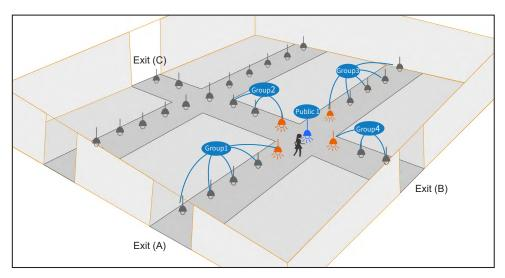
3. When group 3 sensor detect mtion, it will turn on and transfer synchronize signal at the same time, the group3 sensors will turn on and the near by public sensor 1 will trigger and turn on, but it will not transfer synchronze signal to others, those sensors near by the public sensor1 will not turn on.
