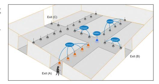
2. When the public sensor detect motion directly, it will transfer the synchronize signal one time only, you can see the sensor near by the public1 will turn on but those next will not.
