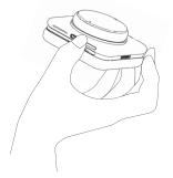
Long press the power button until the indicator light starts blinking, then wait for it to turn solid green. (Notice: Blue indicator light means the Computing Unit is in Sleep Mode. Press the power button to wake it up.)
