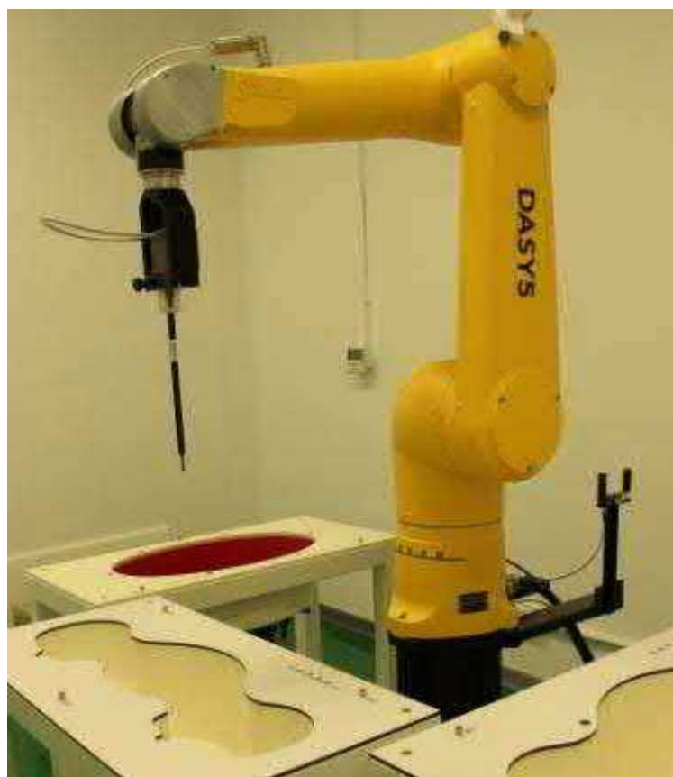
Picture 8.4-1: Specific Absorption Rate Test Layout
